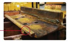
Centered T-Bar welded in the center of the trailing edge.
