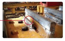
Centered T-Bar with tungsten carbide overlay for additional wear life.
